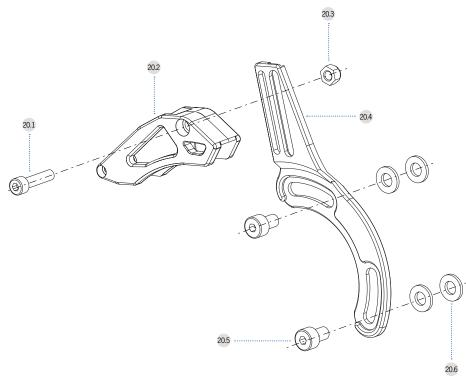
Install 2,5mm worth of washers on each bolt to separate the chainguide bracket from the motor
