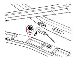
To seat tube. Exits next to charging port and internally through left chainstay.
