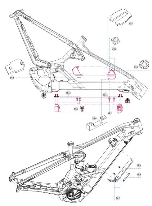
The complete external battery connection kit is only available as an option when purchasing a Wild FS from Orbea For bikes that were purchased with the internal battery only, orbea will facilitate the components that are Orbea's own and specific to the wild fs frame for the installation of the external battery. These items are included in the kit Y0000218 below.
