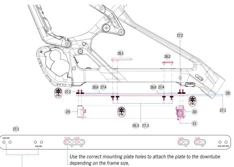
Assemble the PowerTube battery lower holder in its correct position depending on
