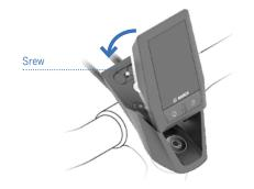
To remove the Kiox display from the OC Components holder, unscrew first the bolt on the back of the holder with a 2.5mm Allen key.
