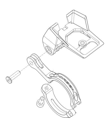
OC COMPONENTS KIOX DISPLAY HOLDER 35MM CARBON: YES | HYDRO: YES
